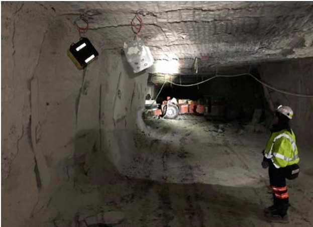
Figure 1. Wireless gas monitors are easily installed in working areas without cables and remain operational even during power outages.
