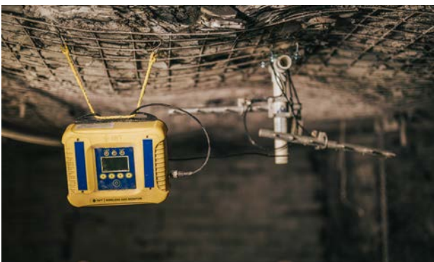
Figure 3. Monitors that offer both internal and external antenna options ensure gas data is transmitted from anywhere in the mine.
