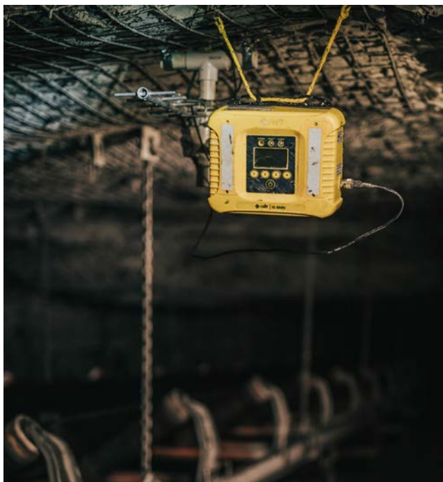
Figure 3. IWT's battery-operated, wireless mesh node allows for fast deployment and enables communications in the working section.
