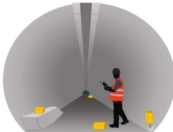
Figure 2: Temporary node installation for short term projects using the ground, outcrops or existing holes
